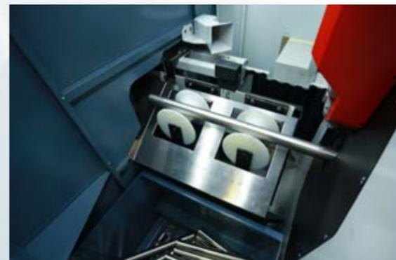
For smaller parts than 800 mm, unloading table stays in outside and another small unloading system unloads the parts.
