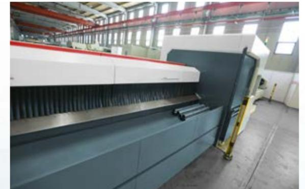
For longer parts than 800 mm, unloading table enters the cabin and unloads the parts.
