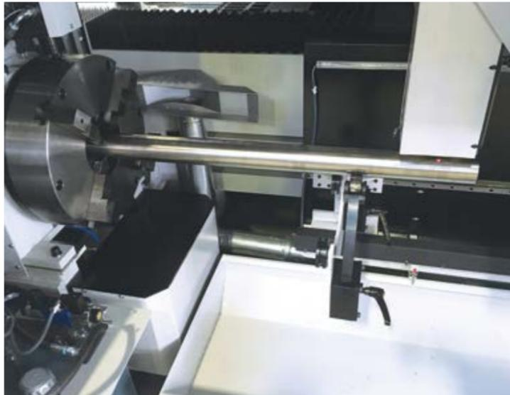
Pipe and tube profile rotation system
